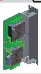
The QE20-FP2023 2 x 4way Splitter Module can be used to split 2 QE20 amplifier 100V outputs into sets of 4, or 1 amplifier 100V output into 8, short circuit isolated 100V loudspeaker feeds for different areas of an evacuation zone, or as a replacement for an existing module.
